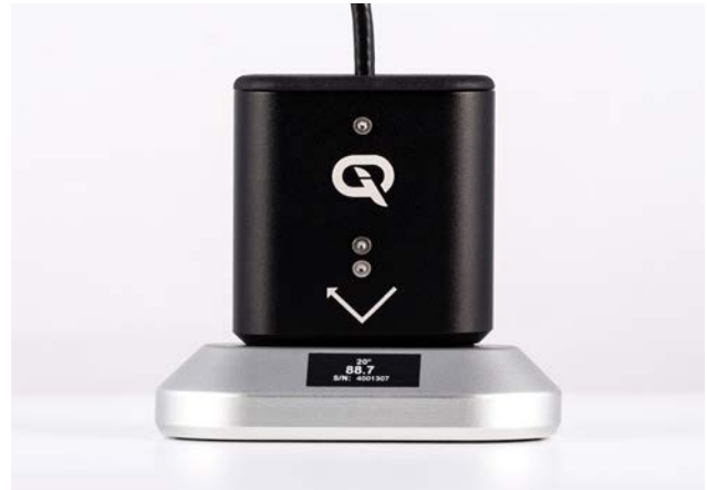
IQ Flex 20 with calibration tile
